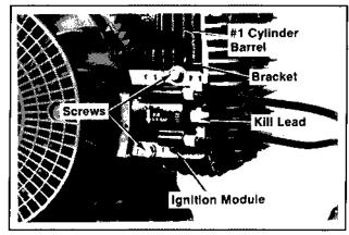
Figure 8-5. Removing Ignition Module.
