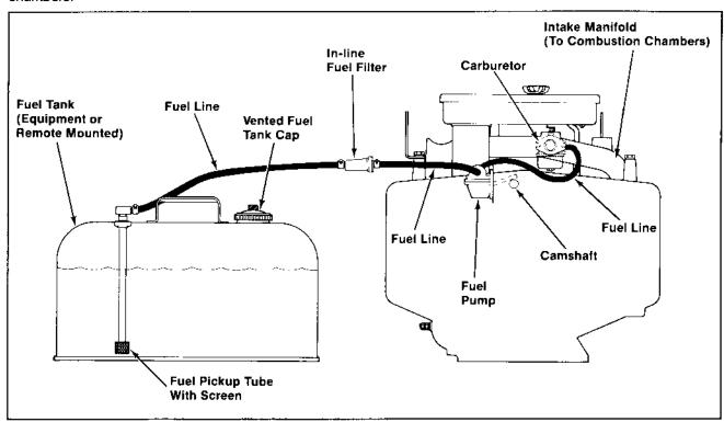
Figure 6A-1. Typical Fuel System.
