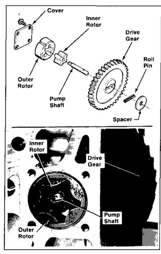
Figure 7-2. Oil Pump Assembly.
