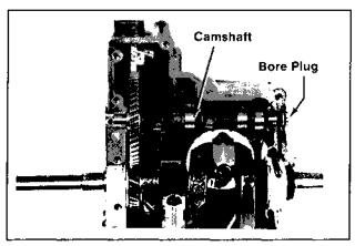
Figure 9-33. Removing The Camshaft and Camshaft Bore Plug.
