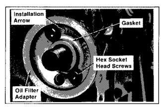
Figure 11-25. Installing Oil Filter Adapter.
