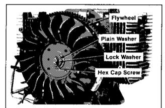
Figure 11-37. Installing Flywheel Fastener.
