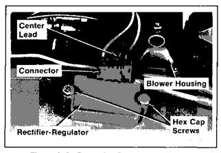
Figure 9-9. Removing Rectifier-Regulator.
