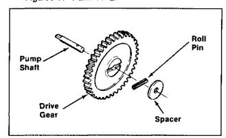
Figure 11-1. Installing Oil Pump Drive Gear.
