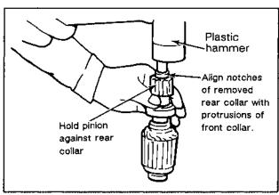
Figure 8-27. Removing the Front Stop Collar.
