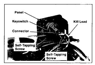
Figure 11-44. Installing Key Switch.
