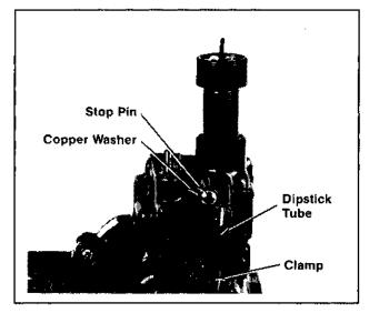
Figure 11-9. Installing Governor Stop Pin.
