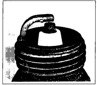
Chalky White Deposits: Chalky white colored deposits indicate overheating. This condition is usually accompanied by excessive gap erosion. A clogged grass screen, clogged cooling fins, and lean carburetion are some causes of overheating.
