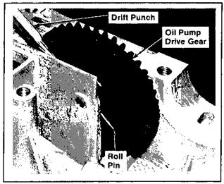
Figure 9-41. Removing Oil Pump Drive Gear.
