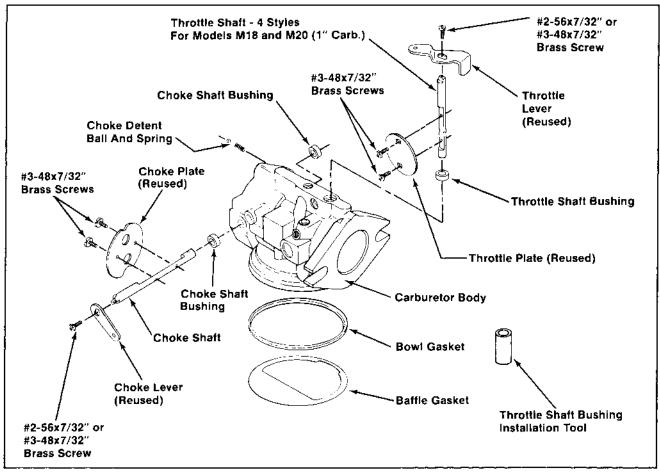
Figure 6A-8. Throttle and Choke Shaft Replacement Kits.
