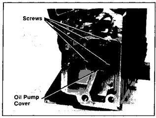
Figure 9-39. Removing Oil Pump Cover.
