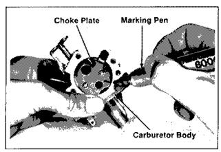
Figure 6B-8. Marking Choke Plate and Carburetor Body.
