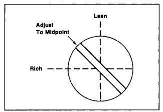
Figure 68-48. Optimum Low Idle Fuel Setting.
