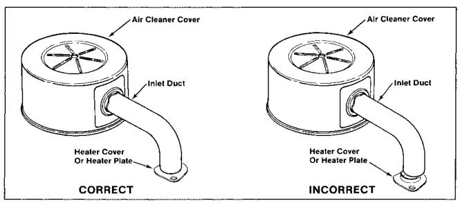
Figure 5-6. Installing Anti-Icing Air Cleaner Cover.
