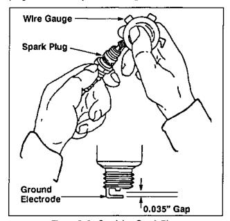
Figure 8-8. Servicing Spark Plug.
