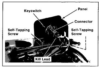
Figure 9-10. Removing Key Switch.
