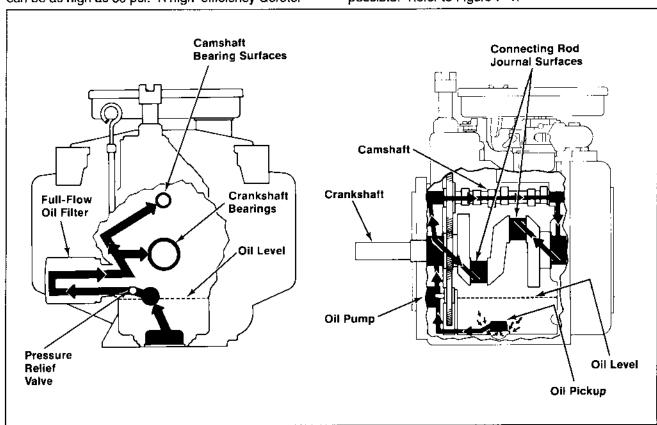
Figure 7-1. Full-Pressure Lubrication System.
