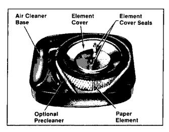
Figure 5-1. Air Cleaner Components.
