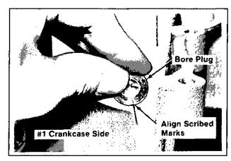
Figure 11-19. Installing Camshaft Bore Plug.
