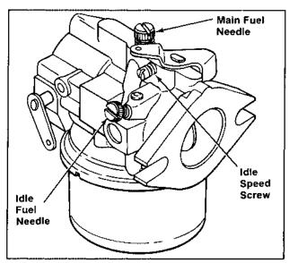
Figure 6A-5. Kohler-Built Adjustable Jet Carburetor.
