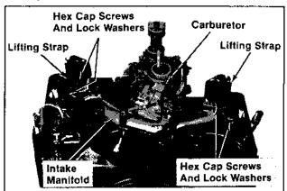
Figure 11-47. Installing Intake Manifold and Carburetor.
