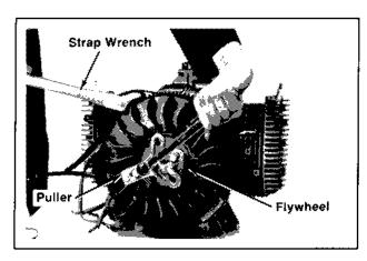
Figure 9-18. Removing Flywheel Using A Puller.
