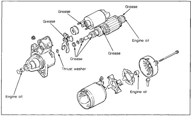
Figure 8-34. Lubrication Points.
