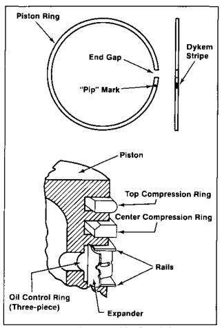
Figure 10-15. Piston Ring Installation.
