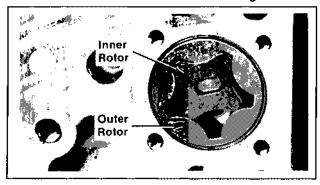
Figure 11-4. Installing Oil Pump Rotors.
