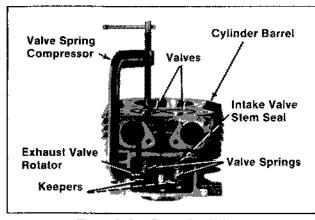
Figure 9-25. Removing Valves.
