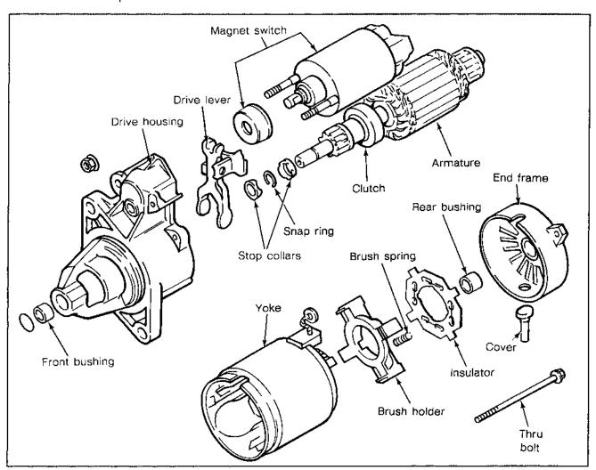
Figure 8-21. Exploded View of Nippensenso Solenoid Shift Starter.
