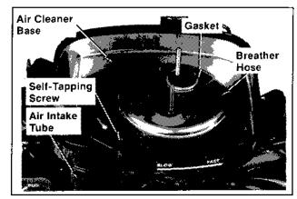
Figure 11-50. Installing Air Cleaner Base.
