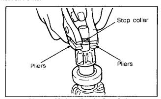
Figure 8-36. Installing the Stop Collar.
