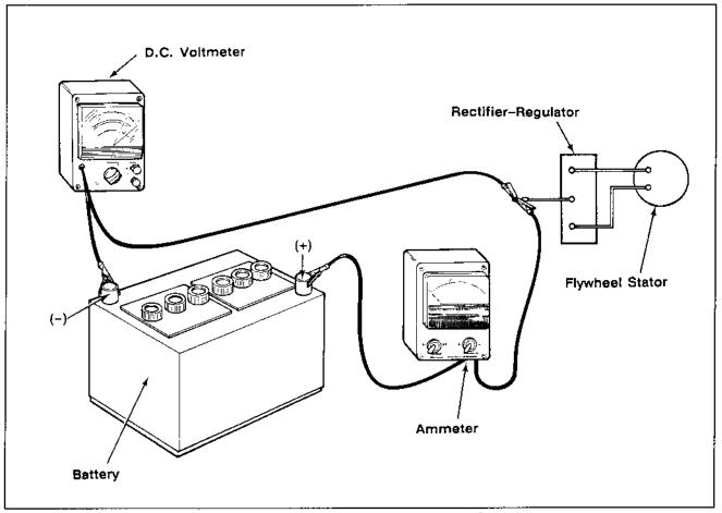
Figure 8-13. Connections for Testing 15 and 25 Systems.
