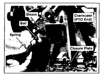
Figure 7-4. Oil Pressure Relief Valve.
