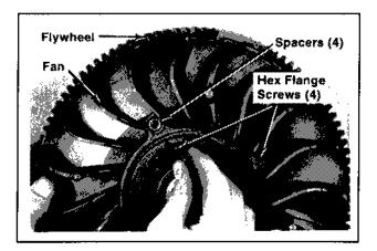
Figure 9-19. Removing Fan From Flywheel.
