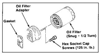
Figure 7-6. Installation Torques— Engine Mounted Oil Filter.
