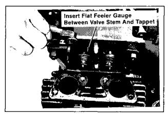
Figure 11-32. Measuring Valve-to-Tappet Clearance.
