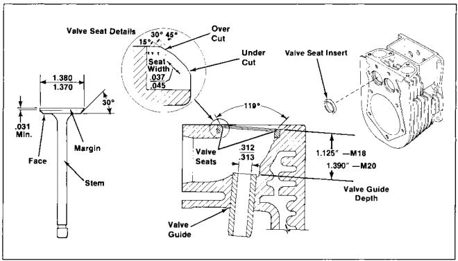
Figure 10-5A. Exhaust Valve Details (30° Angle).
