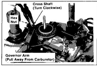
Figure 11-49. Adjusting Governor Arm/Cross Shaft.
