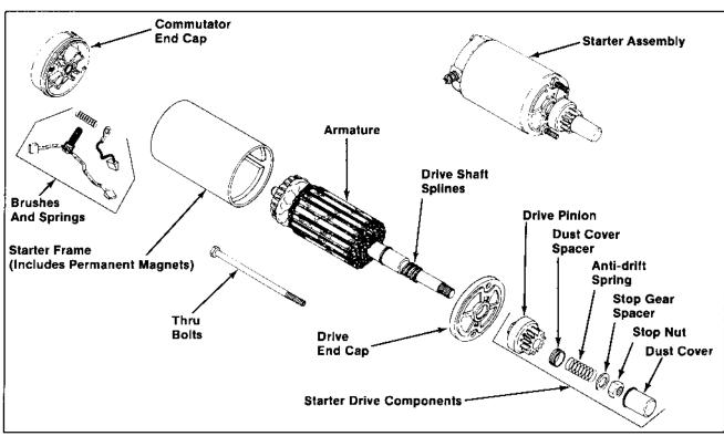
Figure 8-17. Bendix Drive Electric Starter.
