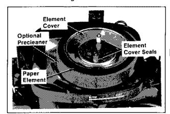
Figure 11-51. Installing Air Cleaner Element.
