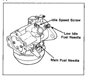
Figure 6B-3. Walbro Adjustable Main Jet Carburetor.
