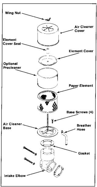
Figure 5-3. Dome Air Cleaner Assembly.
