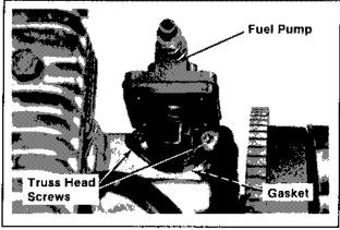
Figure 9-14. Removing Fuel Pump.
