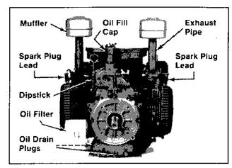
Figure 9-1. Removing Spark Plug Leads, Oil Drain, Oil Filter, and Mufflers.
