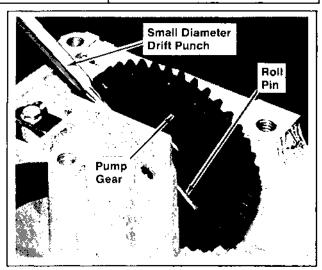
Figure 10-19. Removing the Oil Pump Gear.
