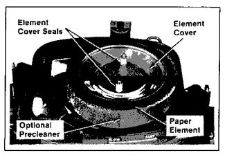
Figure 9-4. Removing Air Cleaner Element.
