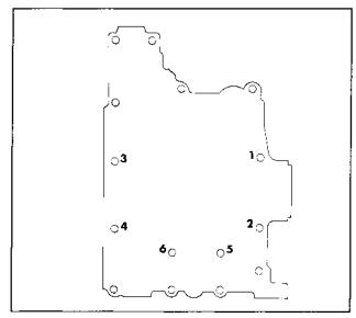
Figure 11-21. Crankcase Fastener Torque Sequence.
