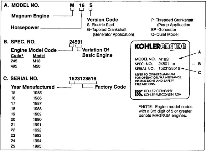
Figure 1-2. Engine Identification Decals.
