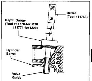
Figure 10-7. Installing Valve Guide.
