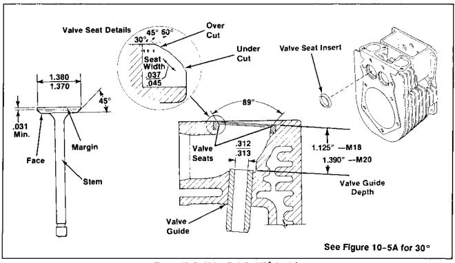
Figure 10-5. Valve Details (45° Angle).
