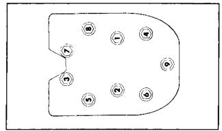
Figure 3-10. Cylinder Head Fastener Tightening Sequence.
