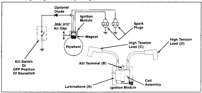
Figure 8-1. Magnum Electronic Magneto Ignition System.
