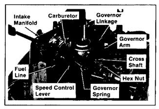
Figure 9-6. Removing Governor Arm, Carburetor, and Intake Manifold.
