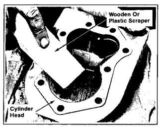
Figure 3-9. Cleaning Cylinder Heads and Combustion Chambers.
