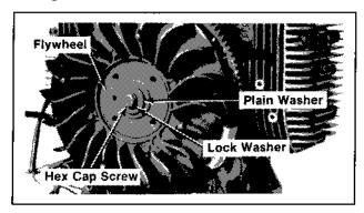
Figure 9-17. Removing Flywheel Fastener.
