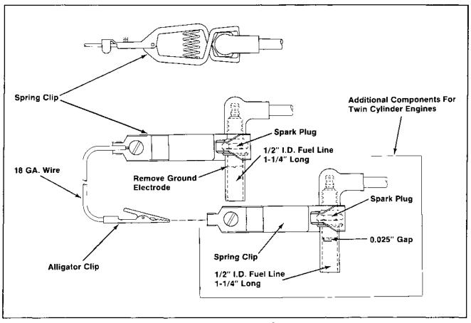
Figure 2-3. Electronic Ignition System Tester.
