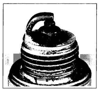
**Wet Fouled:\*** A wet plug is caused by excess fuel, or oil in the combustion chamber. Excess fuel could be caused by operating the engine with too much choke. Oil in the combustion chamber is usually caused by worn piston rings or valve guides.
