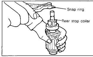
Figure 8-33. Installing Snap Ring.
