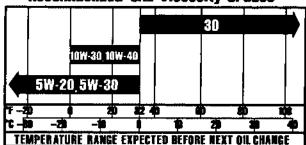
Straight 30-weight oil is preferred. SAE 10W-30 and 10W-40 are not recommended above 32°F (0°C). Using these oils substantially increases oil consumption and combustion chamber deposits.
