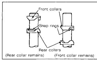
Figure 8-25. Removing the Stop Collar (2).
