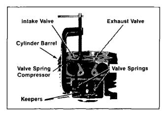
Figure 11-33. Installing Valves. Side #2 Shown.
