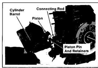
Figure 11-31. Installing Pistons/Cylinder Barrels to Connecting Rod.
