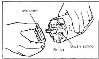
Figure 8-22. Removing the Insulator.
