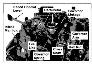
Figure 11–48. Installing Intake Manifold, Carburetor, and Governor Arm.
