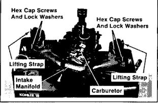
Figure 9-7. Removing Intake Manifold and Carburetor.
