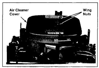
Figure 9-3. Removing Air Cleaner Cover.
