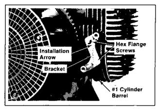
Figure 11-38. Installing Ignition Module Bracket.
