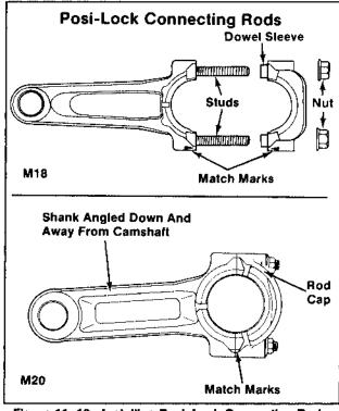
Figure 11-10. Installing Posi-Lock Connecting Rods.
