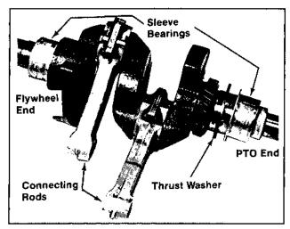
Figure 11-11. Installing Thrust Washer and Bearings to Crankshaft.
