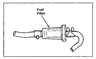
Figure 6A-2. In-Line Fuel Filter.
