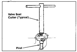
Figure 10-10. Standard Valve Seat Cutter.
