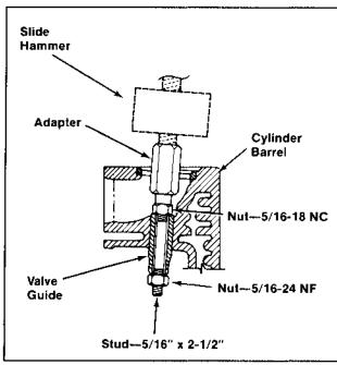
Figure 10-6. Pulling Valve Guide.
