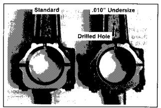
Figure 10-17. Standard and .010" Undersize Service Connecting Rods.
