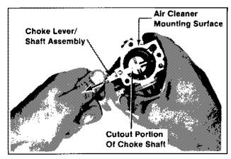
Figure 6B-9. Removing Choke Lever/Shaft.
