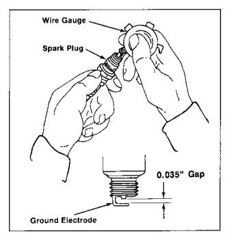
Figure 3-6. Servicing Spark Plugs.
