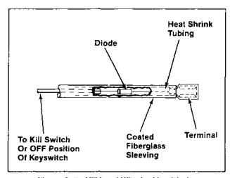
Figure 8-7. Kill Lead With In-Line Diode.
