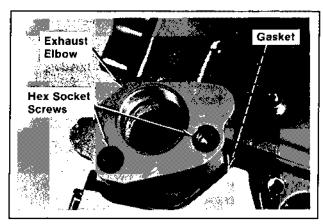
Figure 9-2. Removing Exhaust Elbows.
