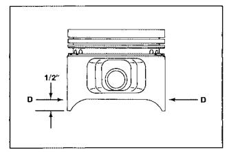
Figure 10-4. Measuring Piston Diameter (Style "D" Piston)
