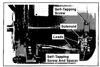
Figure 11-43. Installing Starter Solenoid.
