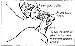
Figure 8-24. Removing the Stop Collar (1).
