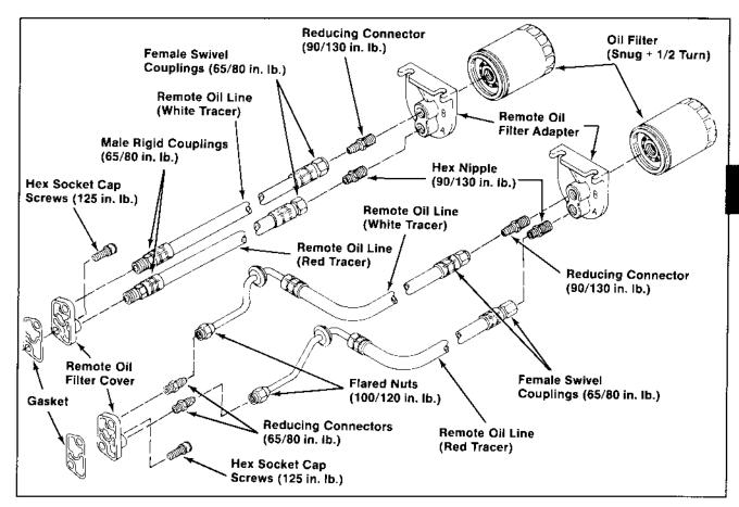
Figure 7-8. Installation Torques--Remote Mounted Oil Filters.
