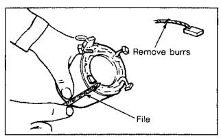
Figure 8-30. Filing Off Burrs on Posts.
