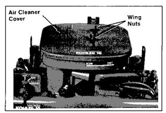
Figure 11-52. Installing Air Cleaner Cover.
