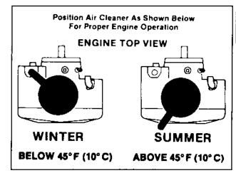
Figure 5-5. Typical Decal - Anti-Icing Air Cleaner Cover Positions.
