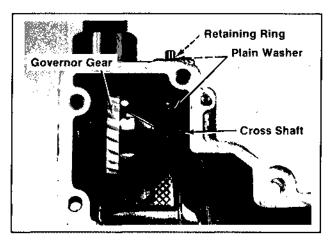
Figure 9-37. Removing Governor Gear.
