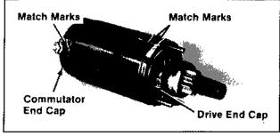
Figure 8-20. Starter Assembly Match Marks.
