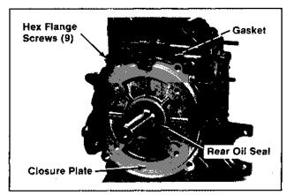
Figure 9-28. Removing Closure Plate.
