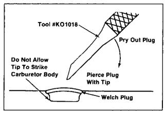
Figure 6B-6. Removing Welch Plugs.
