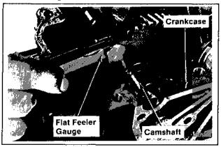
Figure 11-17. Measuring Camshaft End Play.
