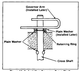
Figure 11-7. Installing Governor Cross Shaft.
