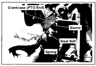
Figure 10-20. Oil Pressure Relief Valve.
