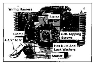
Figure 11-35. Installing Stator and Electric Starter.
