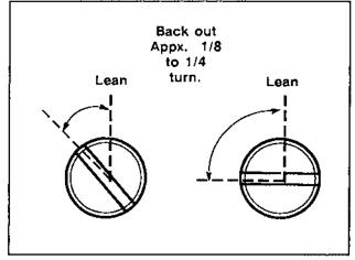
Figure 6B-4A. Optimum Main Fuel Setting.
