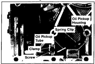
Figure 11-6. Installing Oil Pickup Components.
