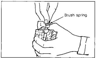
Figure 8-37. Installing the Brush Springs.
