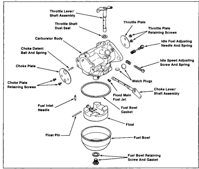
Figure 6B-5. Walbro-Built Carburetor - Exploded View.
