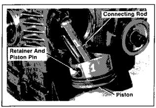
Figure 9-26. Removing Pistons.
