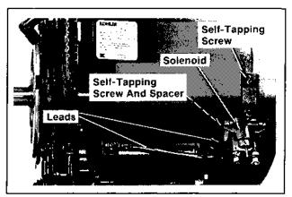
Figure 9-11. Removing Starter Solenold.
