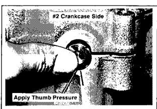
Figure 11-20. Installing #2 Crankcase Side.
