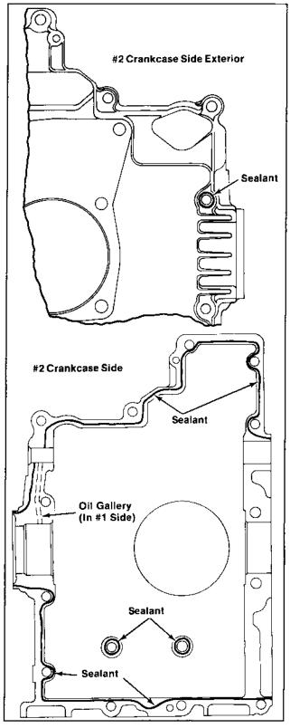
Figure 11-18. Crankcase Sealant Pattern.
