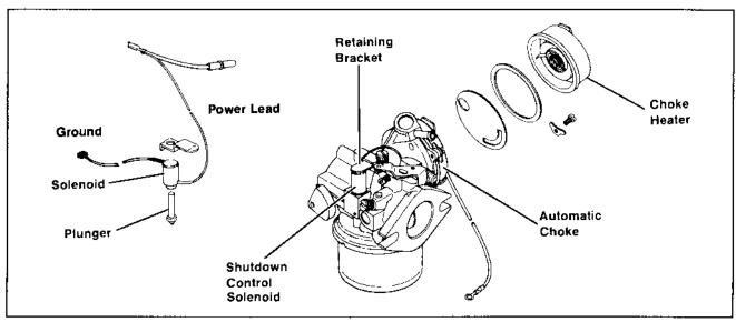
Figure 6A-23. Engine Shutdown Control and Automatic Choke.
