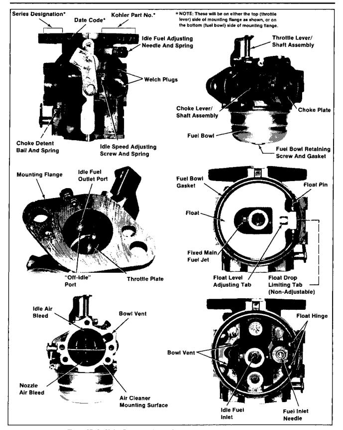
Figure 6B-2. Major Components and Service Locations - Typical Walbro Carburetor.
