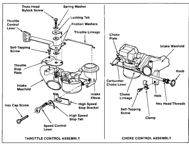
Figure 6A-21. Engine Mounted Throttle and Choke Controls.
