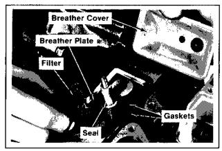
Figure 11-41. Installing Breather Components.
