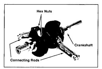
Figure 9-35. Removing Connecting Rods.
