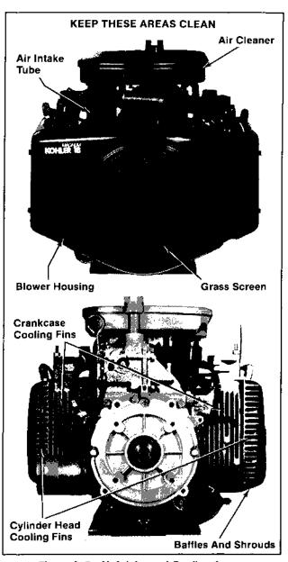
Figure 3-5. Air Intake and Cooling Areas.
