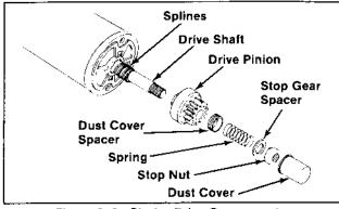
Figure 3-8. Starter Drive Components.
