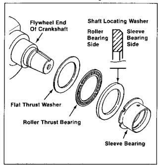
Figure 11-14. Installing Roller Thrust Bearings.
