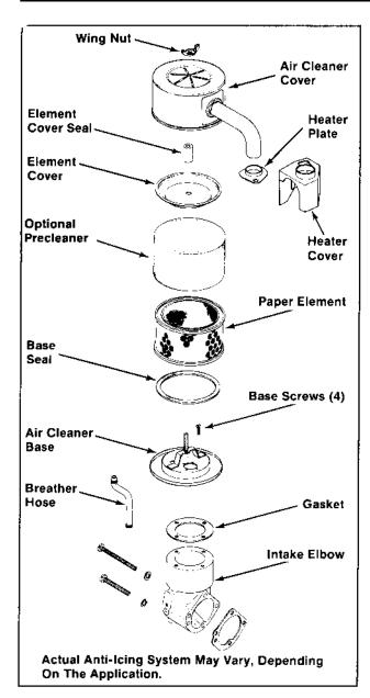
Figure 5-4. Anti-Icing Air Cleaner Assembly.
