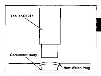
Figure 6B-12. Installing Welch Plugs.
