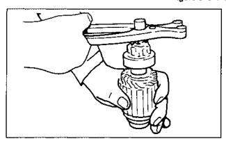
Figure 8-35. Tightening the Snap Ring.
