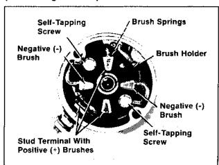
Figure 8-18. Commutator End Cap With Brushes.
