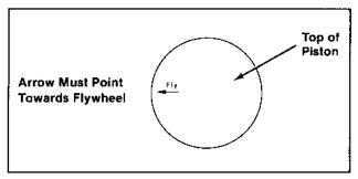
Figure 11-29. Piston Installation Direction Identifier.
