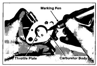
Figure 6B-7. Marking Throttle Plate and Carburetor Body.
