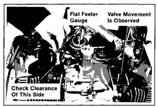
Figure 3-11. Measuring Valve-To-Tappet Clearance.
