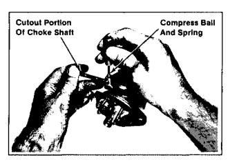
Figure 6B-11. Installing Choke Lever/Shaft.
