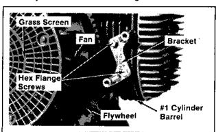
Figure 9-16. Removing Ignition Module Bracket.
