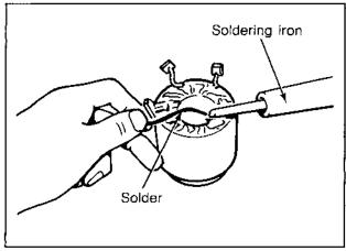
Figure 8-32. Soldering Brush Clips to Posts.
