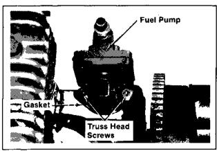
Figure 11-40. Installing Fuel Pump.
