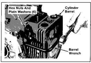
Figure 9-23. Removing Cylinder Barrel Fasteners.
