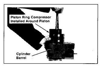
Figure 11-28. Installing Pistons.
