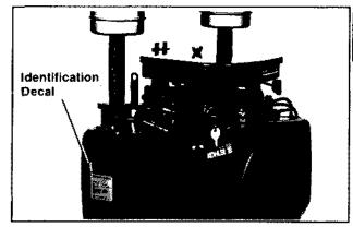
Figure 1-1. Location of Engine Identification Decal.
