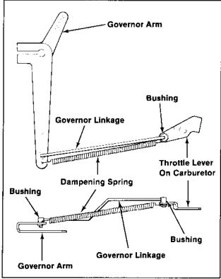
Figure 6B-16. Installing Dampening Spring -- M20 Engines.
