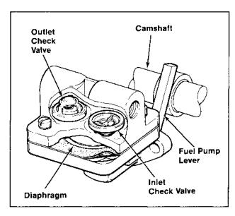
Figure 6A-3. Mechanical Fuel Pump.
