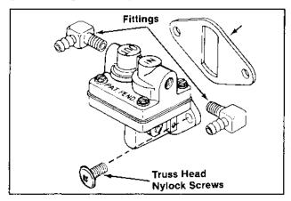
Figure 6A-4. Installing Fuel Pump.
