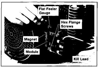
Figure 11-39. Installing Ignition Module.
