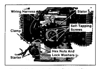
Figure 9-20. Removing Electric Starter and Stator.
