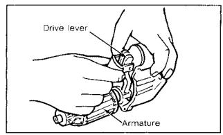
Figure 8-23. Removing the Armature and Drive Lever.
