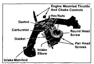
Figure 11-46. Installing Carburetor to Intake Manifold.
