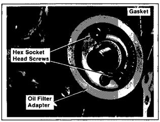
Figure 9-30. Removing Oil Filter Adapter.
