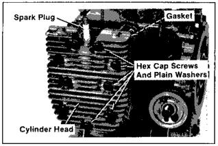
Figure 9–22. Removing Spark Plugs and Cylinder Heads.
