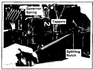
Figure 9-32. Splitting The Crankcase.
