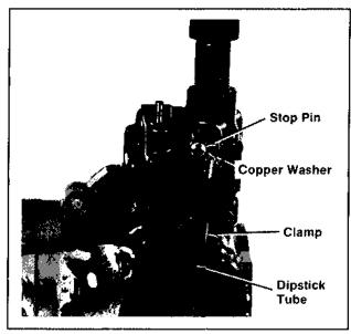
Figure 9-36. Removing Governor Stop Pin.
