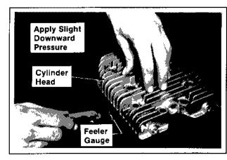
Figure 10-1. Checking Cylinder Head Flatness.
