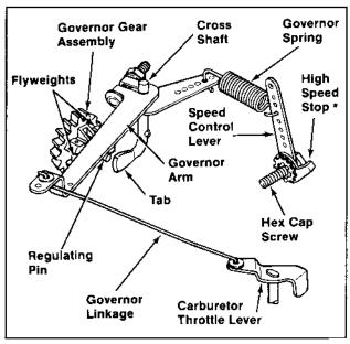
Figure 6A-16. Centrifugal Flyweight Mechanical Governor.
