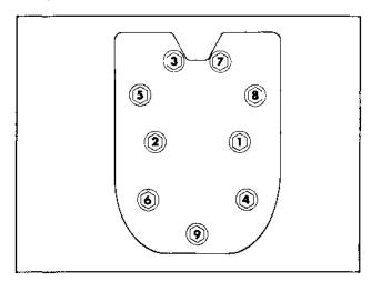
Figure 11-34. Cylinder Head Fastener Torque Sequence.
