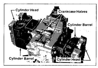
Figure 9-21. Identifying Engine Sides.
