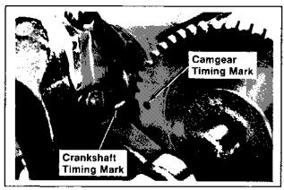
Figure 11–16. Aligning Crankshaft and Cam Gear Timing Marks.
