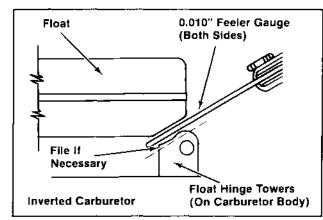
Figure 6A-15. Checking Float Clearance.
