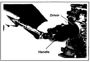
Figure 11-24. Installing Oil Seal Using Driver.
