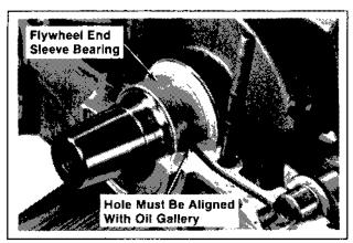
Figure 11-13. Position of Flywheel Bearing.
