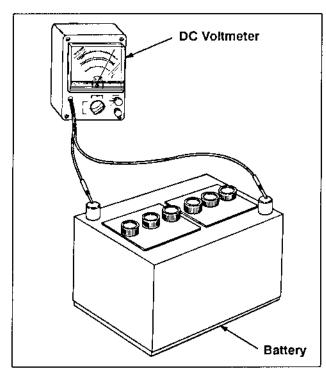
Figure 8-14. Checking Battery Voltage.
