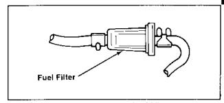
Figure 3-7. In-line Fuel Filter.
