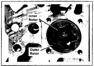
Figure 9-40. Removing Oil Pump Rotors.
