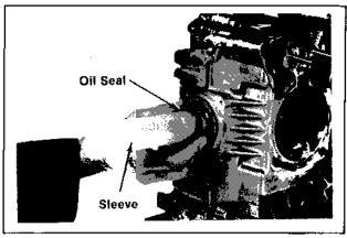
Figure 11-23. Installing Oil Seal Using Sleeve.
