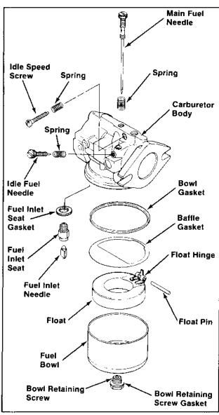
Figure 6A-7. Kohler-Built Adjustable Jet Carburetor - Exploded View.
