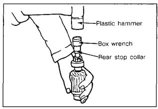
Figure 8-26. Removing the Rear Stop Collar.
