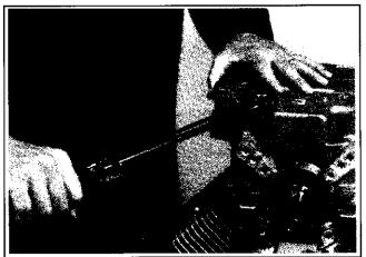
Figure 11-15. Tighten Crankcase Halves to Torque.
