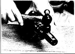
Figure 10-1. Installing Key For Sprocket.
