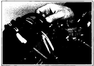
Figure 11-53. Connecting Fuel Line To Carburetor.
