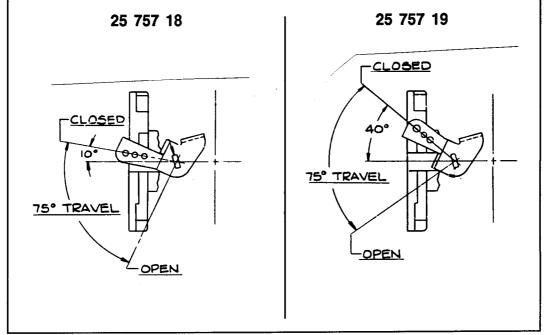
For 1" carburetors determine which kit you need by measuring your throttle shaft as shown below:
